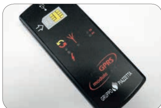
Kit Remote Control System (modulo GPRS per la gestione con SMS) Remote Control System kit (GPRS module for a controlling with SMS)
