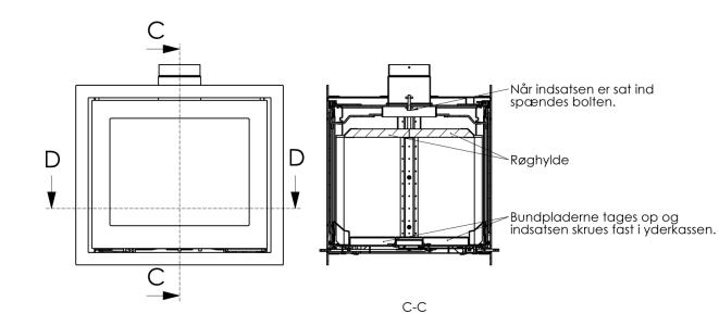
The potential for the building-in of fireplace inserts is vast. Building-in shall take place in connection with non-inflammable materials only. Virtually all installations are designed individually, and in all cases the distance to inflammable matter must meet the values stated below.
