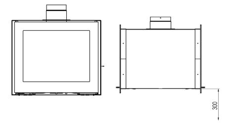
Distance to inflammable material is 500mm to the side, but can be reduced to 60mm by using isolating material like "Isolrath 1000".
