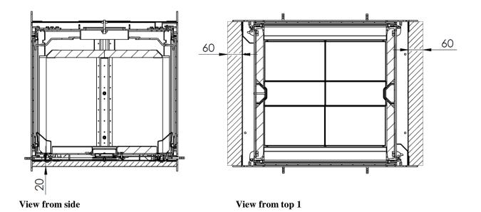
**Insulating material:** Useable are all AGI Q 132 registered insulating material. All measurements are intended as minimum distances.
