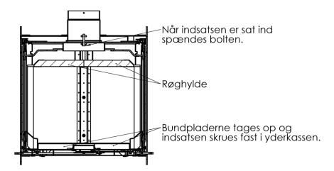
The smoke turn plate is removed by lifting at one side after which it will come clear of the other side and be taken down into the combustion chamber and out through the door. Similarly, it is put in place by moving it up askew at one side and then at the other side, and it is then put in place in the middle.
