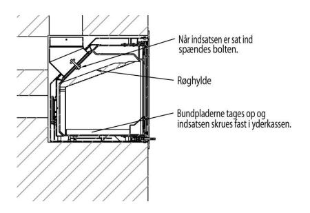
The potential for the building-in of fireplace inserts is vast; they may be built into the wall, on the outside of the wall, and may be suspended on the wall. Building-in shall take place in connection with non-inflammable materials only. Virtually all installations are designed individually, and in all cases, the distance to inflammable matter must meet the values stated below.
