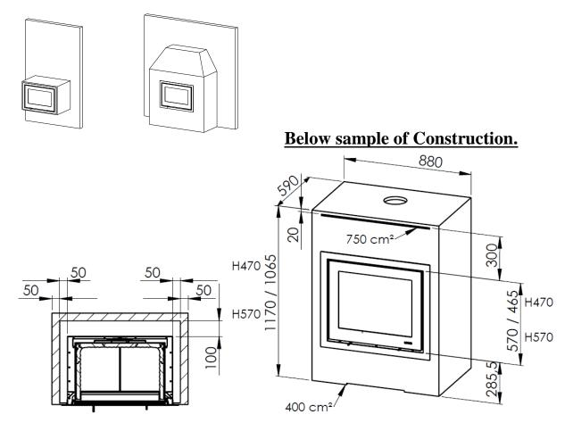
**Insulating material:** Useable are all AGI Q 132 registered insulating material. All measurements are intended as minimum distances.
