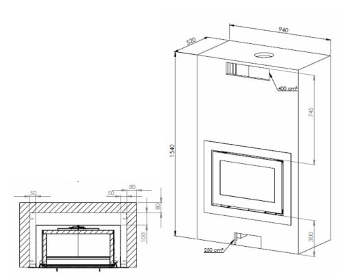
**Insulating material:** Useable are all AGI Q 132 reistered insulating material. All measurements are intended as minimum distances.
