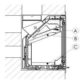
A: upper smoke turnplate-B: lower smoke turnplate C: Skamol (must be removed to get to the screws)
